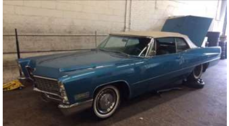
Balancing of rear wheel assemblies required raising of rear-end and chocking opposite wheel
