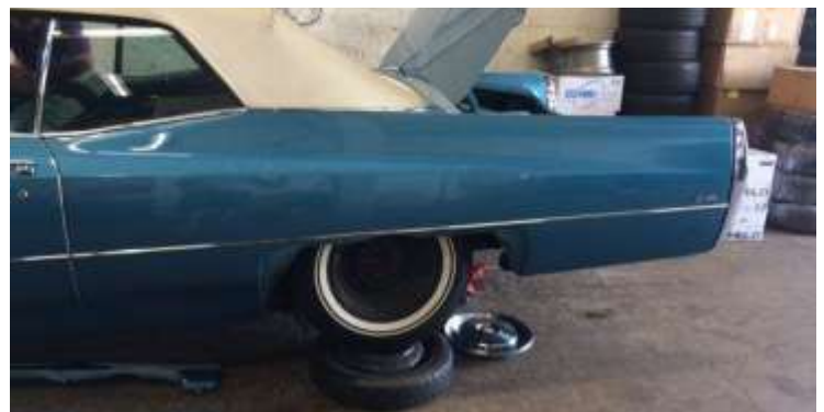
Driver-side Rear wheel chocked while we balanced the passenger side wheel/tire
