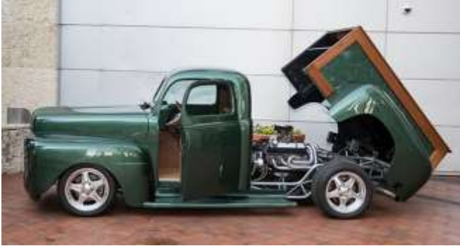
This is a GT40 with a 48 Ford pickup truck built up on top. The ultimate sleeper.
